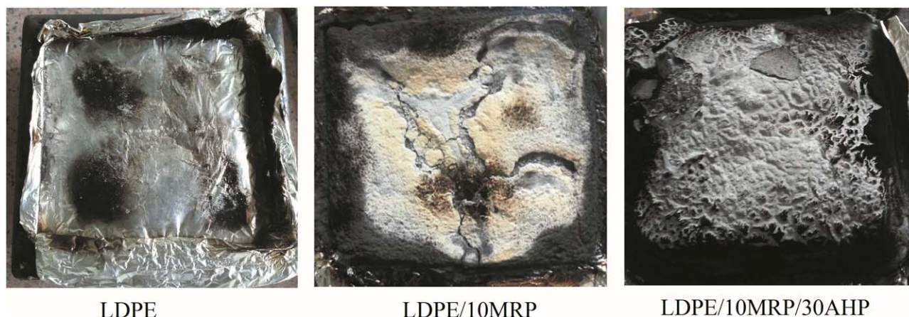
Figure 6. Digital pictures of the residue char after cone calorimetry testing. [Color figure can be viewed in the online issue, which is available at wileyonlinelibrary.com .]
